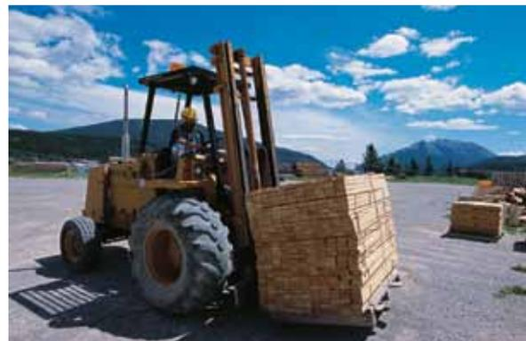
*This forklift is used outdoors for moderate loads of construction material.*
